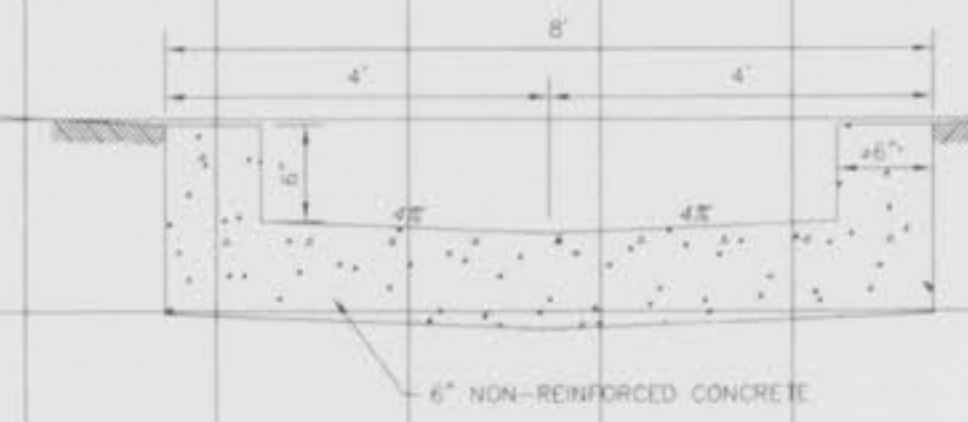
CONCRETE SWALE NOT TO SCALE
