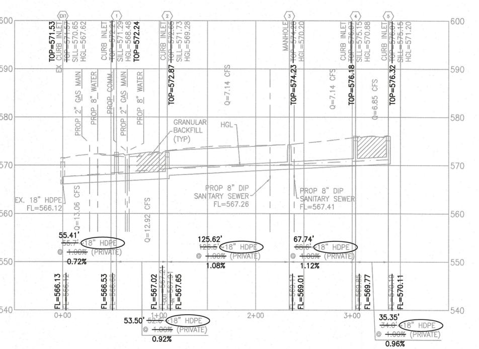
NOTE: COMPACTED GRANULAR TRENCH FILL IS REQUIRED BETWEEN PIPES AT ALL LOCATIONS WHERE WATER MAINS, SANITARY SEWERS, AND STORM SEWERS CROSS OVER EACH OTHER.
