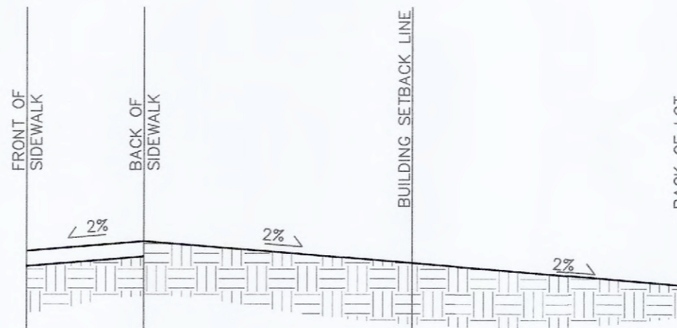
TYPICAL SWALE PROFILE NOT TO SCALE
