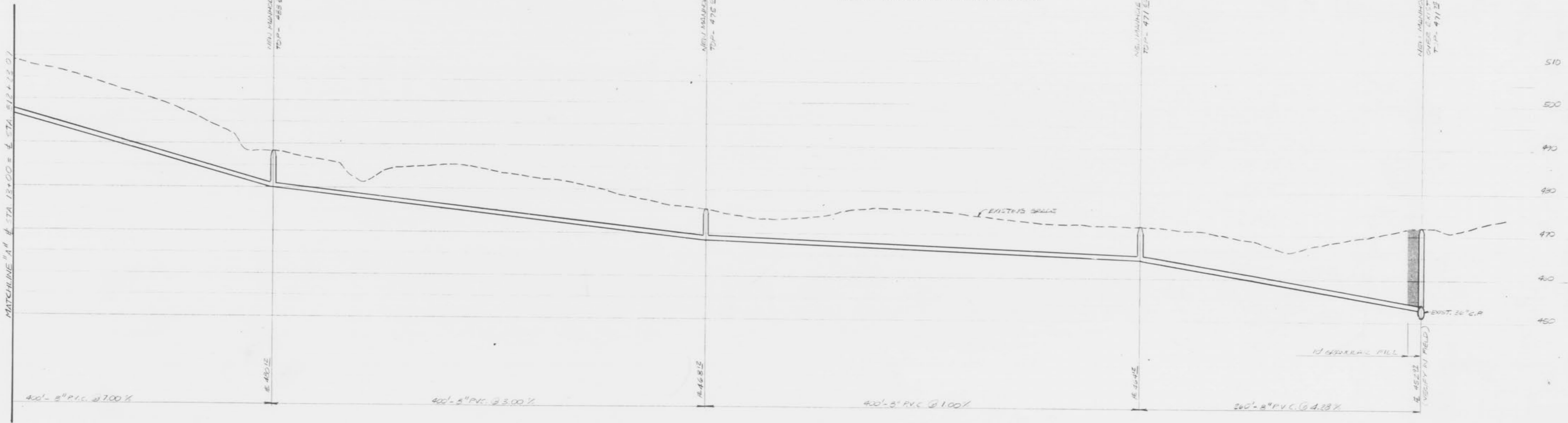
OFF-SITE SANITARY SEWER PROFILE HORIZ. SCALE: 1\"/>
