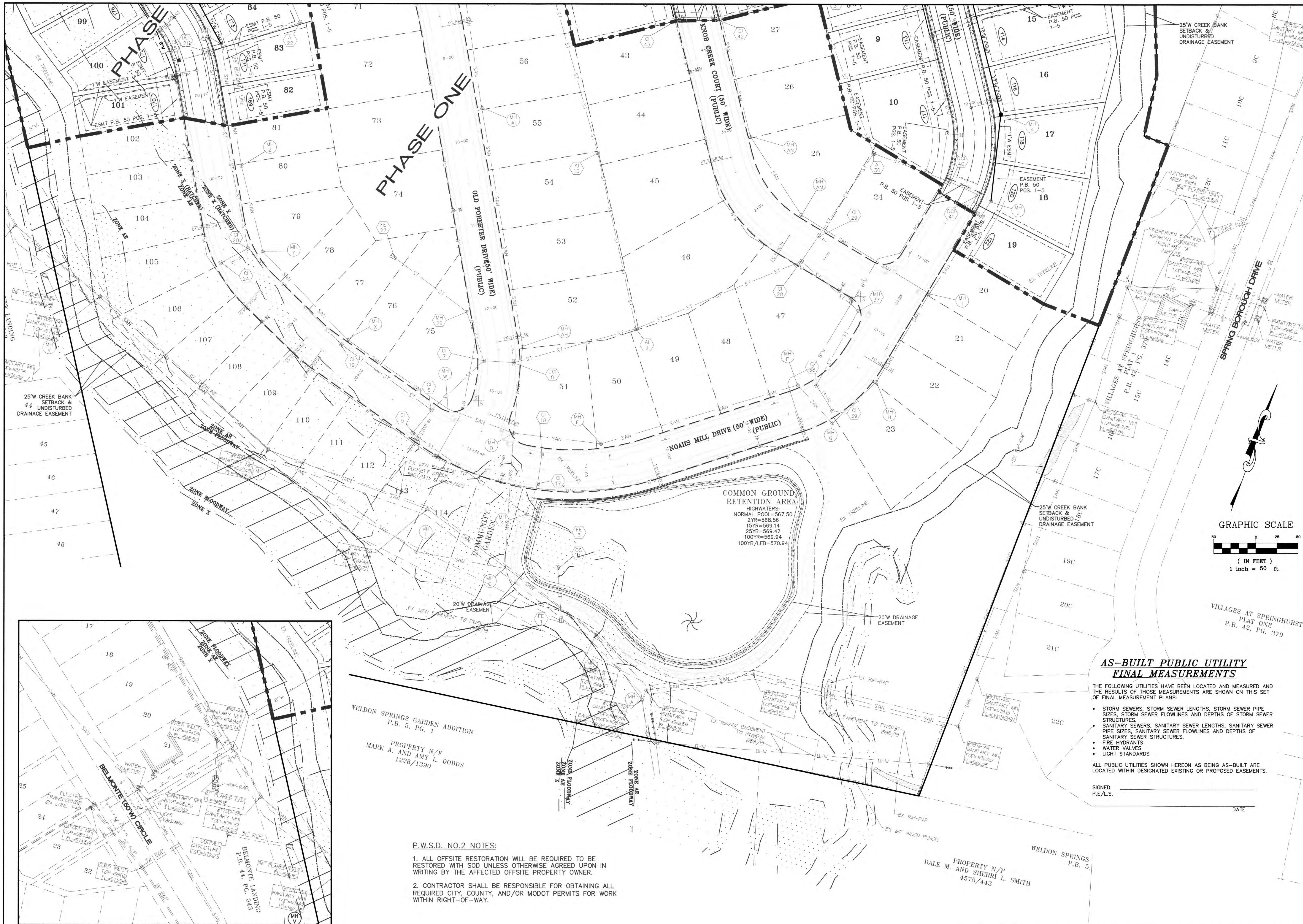
WEST WATER CONNECTION PLAN (SEE SHEET 11A FOR PLAN AND PROFILE)
