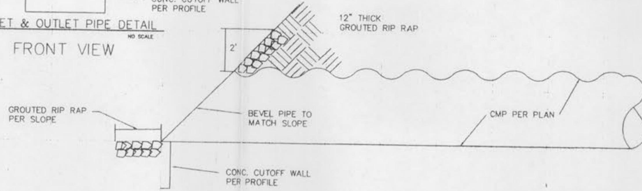
INLET & OUTLET PIPE DETAIL
