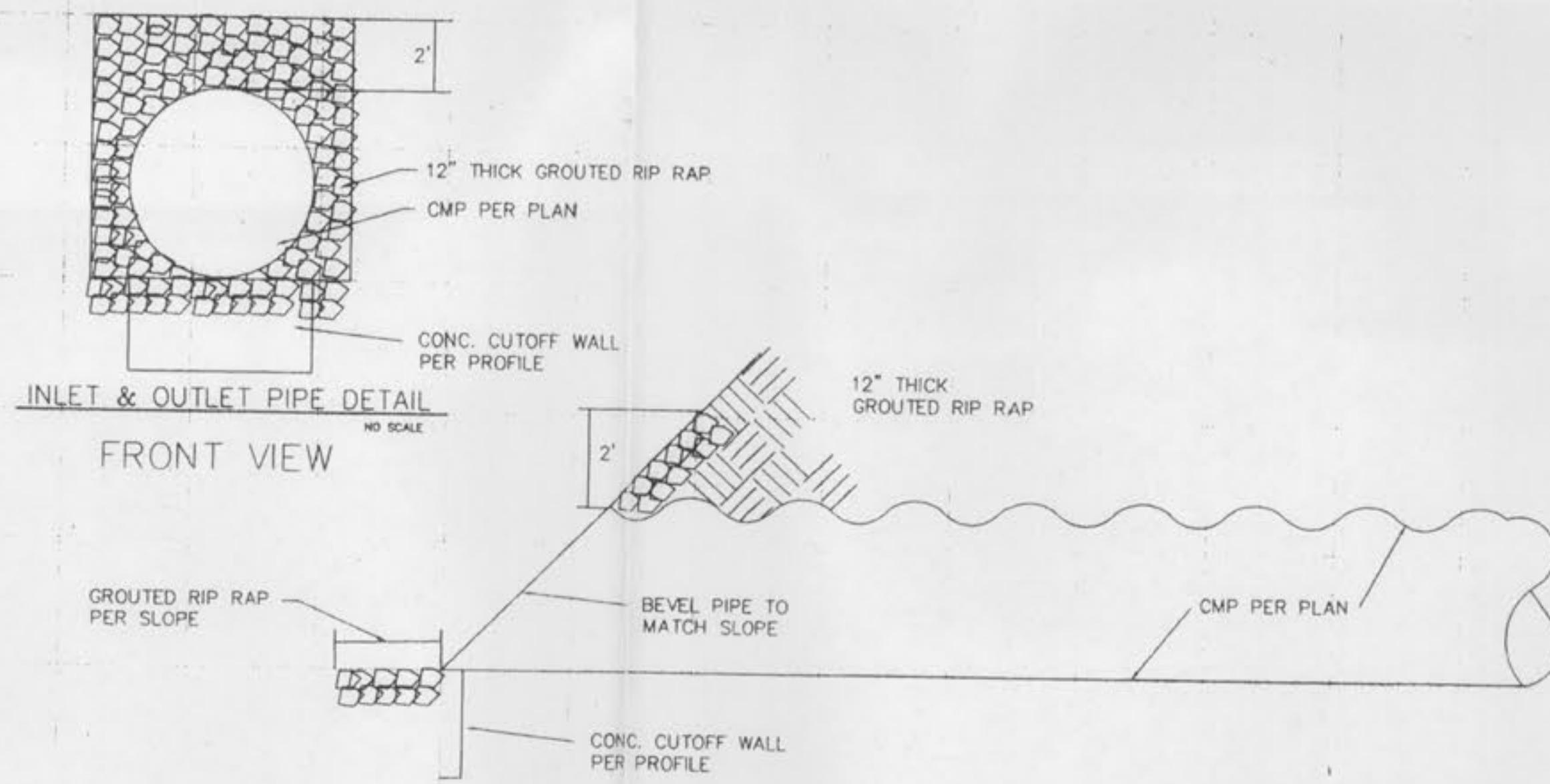
INLET & OUTLET PIPE DETAIL
