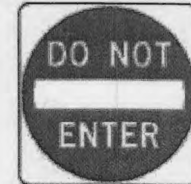
R5-1 30"x30" SIGN PLACED ON HEAVY "U" CHANNEL PAINTED BLACK STEEL POSTS. POSTS TO EXTEND A MINIMUM OF 30" INTO THE GROUND. SIGN TO COMPLY WITH NOTE RN #19 ON SHEET 2. MOUNT BOTTOM OF SIGN A MINIMUM OF 5'-6" ABOVE GRADE.
