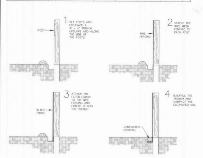
1. FILTER BARRIERS SHALL BE INSPECTED IMMEDIATELY AFTER EACH RAINFALL AND AT LEAST DAILY DURING PROLONGED RAINFALL ANY REQUIRED REPAIRS SHALL BE MADE IMMEDIATELY. 2. SHOULD THE FABRIC DECOMPOSE OR BECOME INEFFECTIVE PRIOR TO THE END OF THE EXPECTED USABLE LIFE AND THE BARRIER
