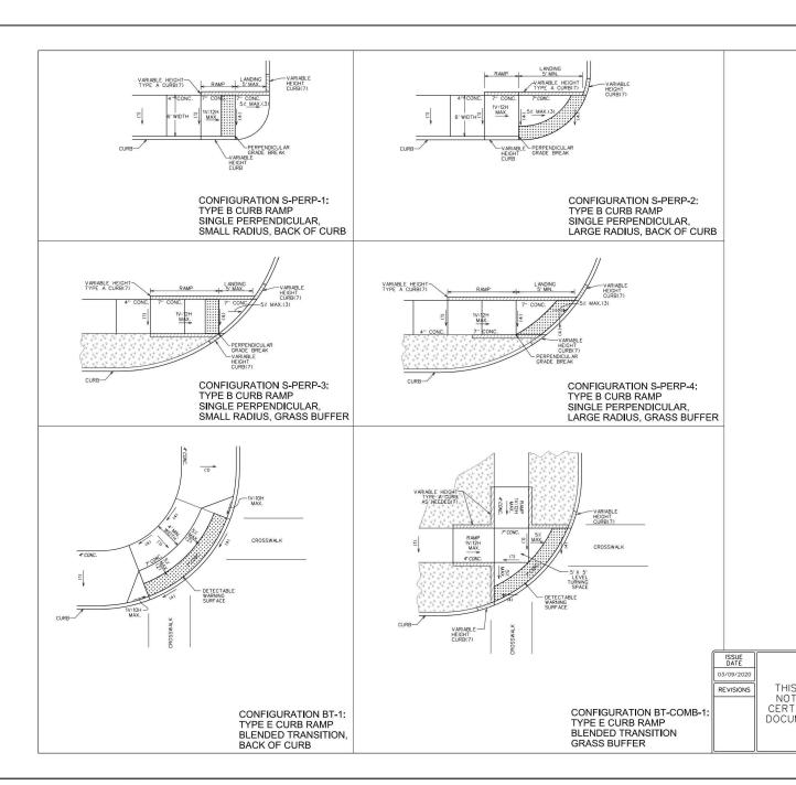
(1) CROSS SLOPE SHALL BE SUFFICIENT TO PREVENT PONDING UP TO A MAXIMUM OF 2% UNLESS OTHERWISE NOTED, 1.5% (+/-)0.5% CROSS SLOPE RECOMMENDED. (2) THE RUNNING SLOPE OF A BLENDED TRANSITION MAY BE WARPED TO MEET ROAD GRADE UP TO 5% MAXIMUM. (3) ALGEBRAIC DIFFERENCE BETWEEN PAVEMENT OR GUTTER SLOPE IN THE DIRECTION OF PEDESTRIAN TRAVEL AND CURB RAMP SLOPE SHALL NOT EXCEED 13.0%. PROVIDE A 24" LEVEL LANDING IF ALGEBRAIC DIFFERENCE EXCEEDS 13.0%.
