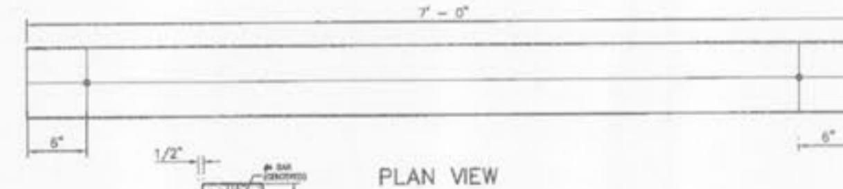
PRECAST CONCRETE WHEELSTOP NOT TO SCALE
