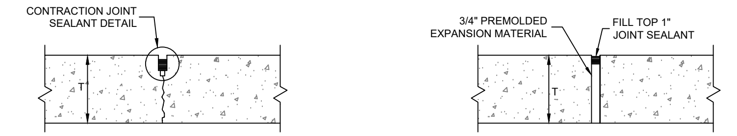
SAWED CONSTRUCTION JOINT
