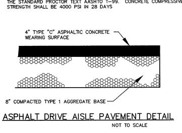
\* ALL GRANULAR ROLLED STONE BASE UNDER PROPOSED CONCRETE MUST BE COMPACTED TO 100% OF THE MAXIMUM DENSITY AS DETERMINED BY THE STANDARD PROCTOR TEXT AASHTO T-99. CONCRETE COMPRESSIVE STRENGTH SHALL BE 4000 PSI IN 28 DAYS
