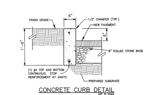
\* ALL GRANULAR ROLLED STONE BASE UNDER PROPOSED CONCRETE MUST BE COMPACTED TO 100% OF THE MAXIMUM DENSITY AS DETERMINED BY THE STANDARD PROCTOR TEXT AASHTO T—99. CONCRETE COMPRESSIVE
