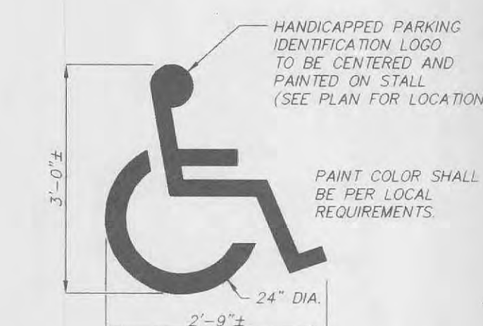
HANDICAPPED PARKING MARKING N.T.S.
