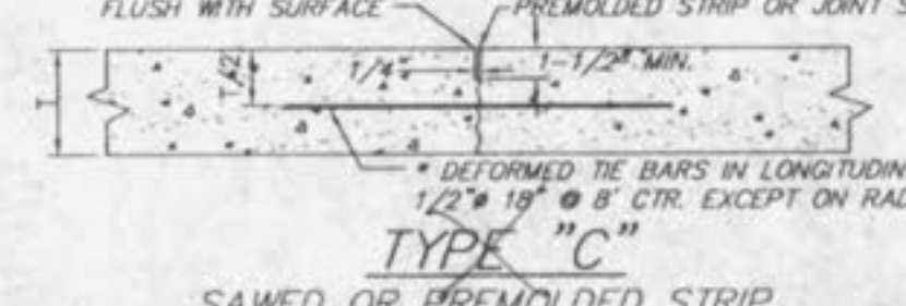
TYPE "C" SAWED OR PREFORMED STRIP LONGITUDINAL OR TRANSVERSE
