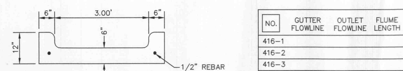
CONCRETE DRAINAGE FLUME 416
