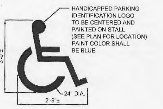
HANDICAPPED PARKING IDENTIFICATION LOGO TO BE CENTERED AND PAINTED ON STALL (SEE PLAN FOR LOCATION) PAINT COLOR SHALL BE BLUE
