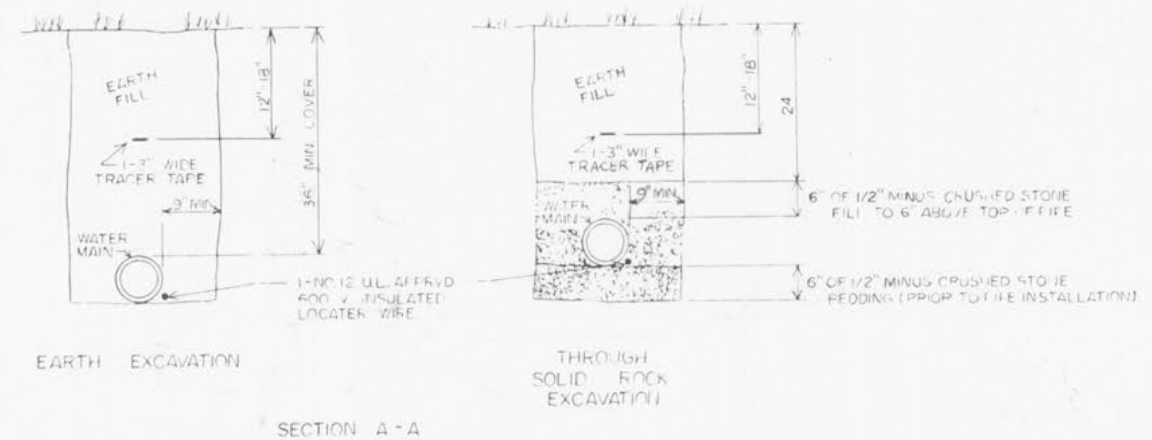
TYPICAL WATER MAIN INSTALLATION DETAILS NO SCALE
