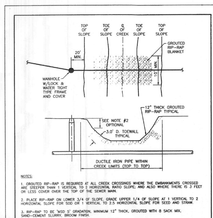
4. INCORPORATE A 3 FEET DEEP TOE WALL ON EMBANKMENT'S UPPER EDGE OF RIP-RAP.
