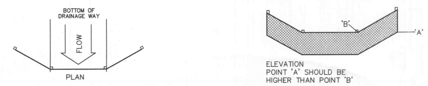
SILTATION FENCE DETAIL NOT TO SCALE
