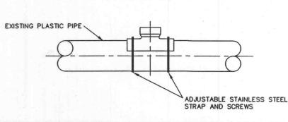
WHEN CONNECTION TO A PLASTIC PIPE IS ALLOWED AND A CONNECTION IS LARGER THAN 6" IN DIAMETER, A SOLVENT WELD OR TEE FITTING OF A SIMILAR MATERIAL MUST BE USED. THIS IS ACCOMPLISHED BY CAREFULLY CUTTING A HOLE WITH A SAW IN THE MAIN AT THE REQUIRED LOCATION AFTER CUTTING AND SHAPING THE HOLE TO THE SIZE OF THE FITTING. THE FOLLOWING STEPS SHOULD BE TAKEN.
