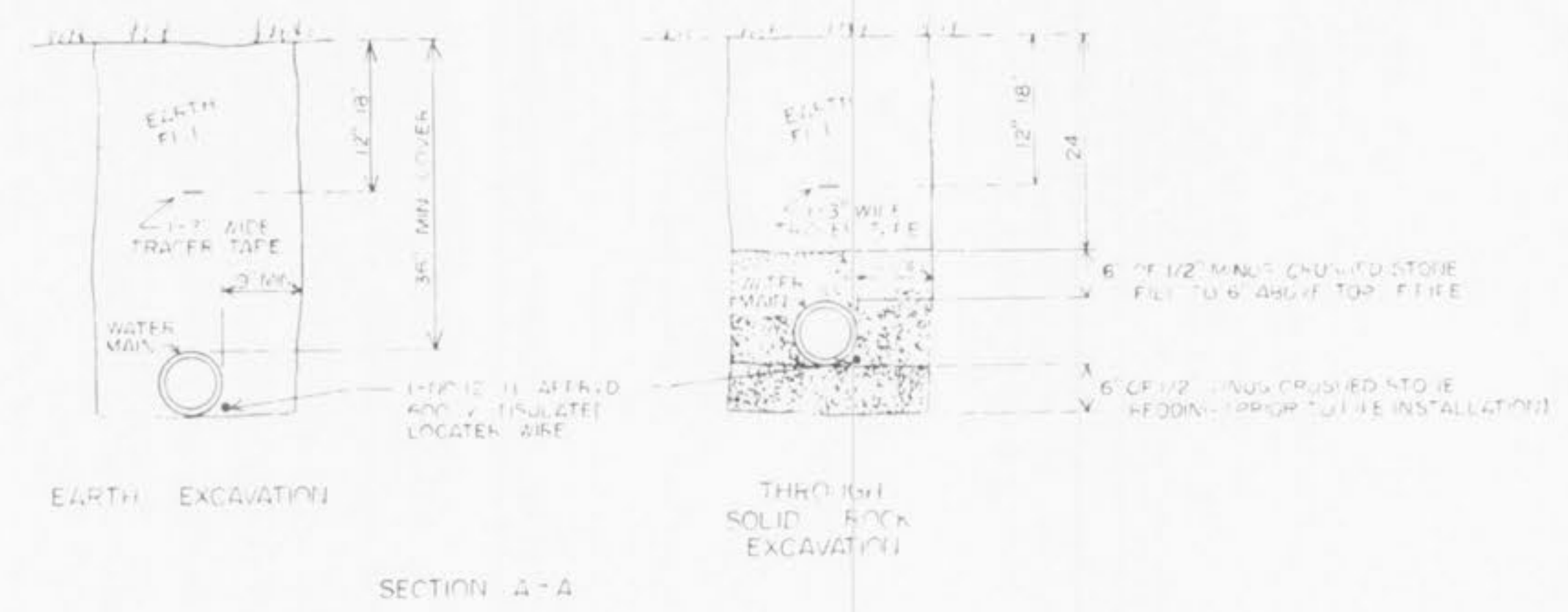
TYPICAL WATER MAIN INSTALLATION DETAILS NO SCALE
