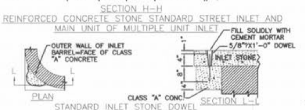
STANDARD - INLET STONES, BLOCKS & DESIGN DETAILS
