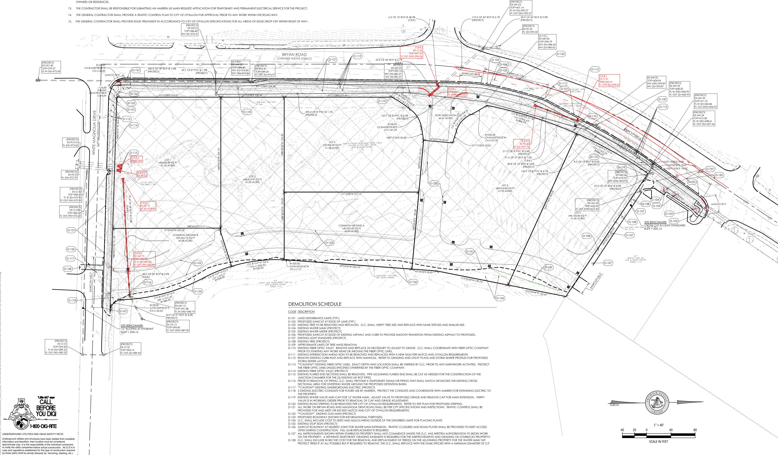
INTENT OF DEMOLITION PLA IT IS THE INTENT OF THIS PLAN THAT ALL REQUIRED DEMOLITION IS COMPLETED AND THE CONTRACTOR SHALL HAVE RENDERED A SITE THAT IS READY FOR CONSTRUCTION. ALL ONSITE FEATURES OBSERVABLE AT THE TIME THE TOPOGRAPHIC SURVEY WAS COMPLETED ARE SHOWN ON THIS PLAN. IF ADDITIONAL REMOVALS ARE REQUIRED, DUE TO CONFLICTING AND OR DIFFERENT CONDITIONS,
