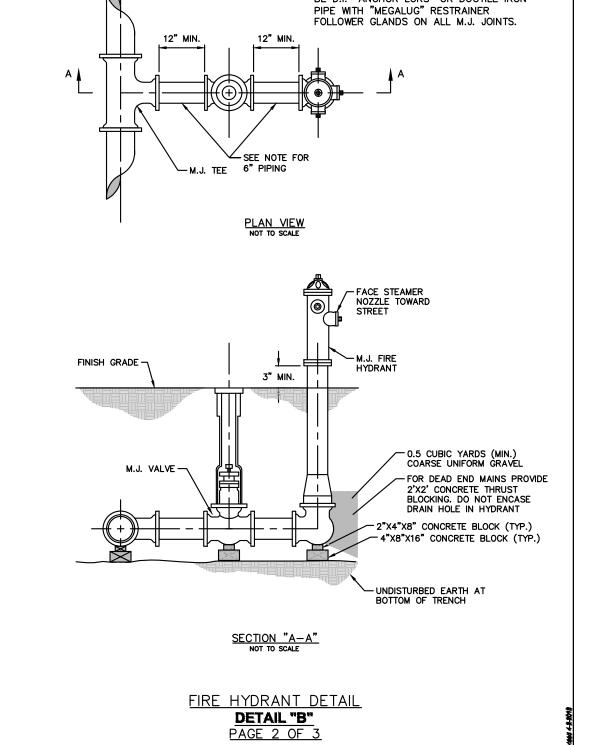
6" PIPES BETWEEN TEE AND VALVE AND BETWEEN VALVE AND FIRE HYDRANT SHALL
