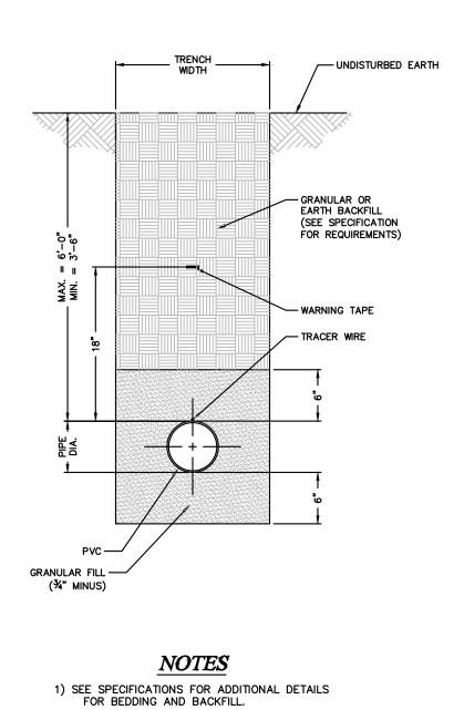
TYPICAL TRENCH SECTION FOR PVC PIPE
