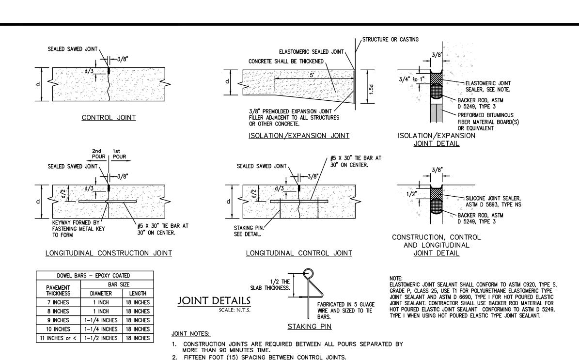
3. FILL JOINTS TO WITHIN 1/8" OF SURFACE WITH JOINT SEALER.
