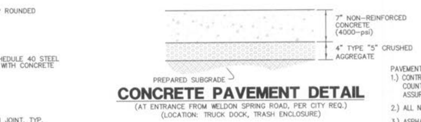
CONCRETE PAVEMENT DETAIL (AT ENTRANCE FROM WELDON SPRING ROAD, PER CITY REQ.) (LOCATION: TRUCK DOCK, TRASH ENCLOSURE)
