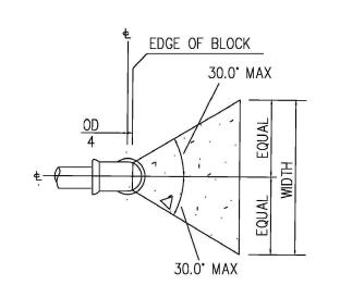
THRUST BLOCK (Plan View)
