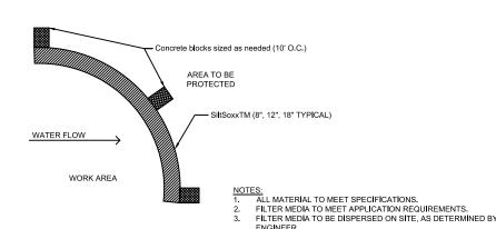
SiltSoxxTM for Sediment Control on Pavement
