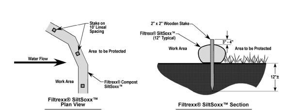
. All material to meet Filtrexx® specifications. SiltSoxx™ compost/isoil/rock/seed fill to meet application 3. SiltSoxx™ depicted is for minimum slopes. Greater slopes may require larger socks per the Engineer. 4. Compost material to be dispersed on site, as determined by Engineer
