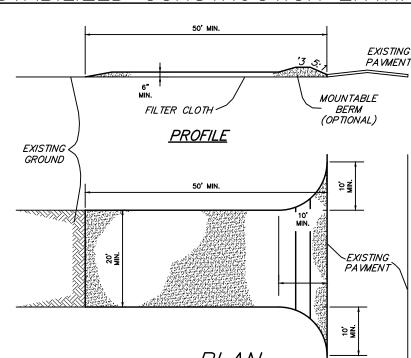
CONSTRUCTION SPECIFICATIONS 1. Stone Size - Use 2" stone, or reclaimed or recycled concrete equivalent. 2. Length — As required, but not less than 50 feet (except on a single residence lot where a 30 foot minimum length would apply).
