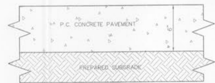
TRASH ENCLOSURE PAVEMENT DETAIL NOT TO SCALE
