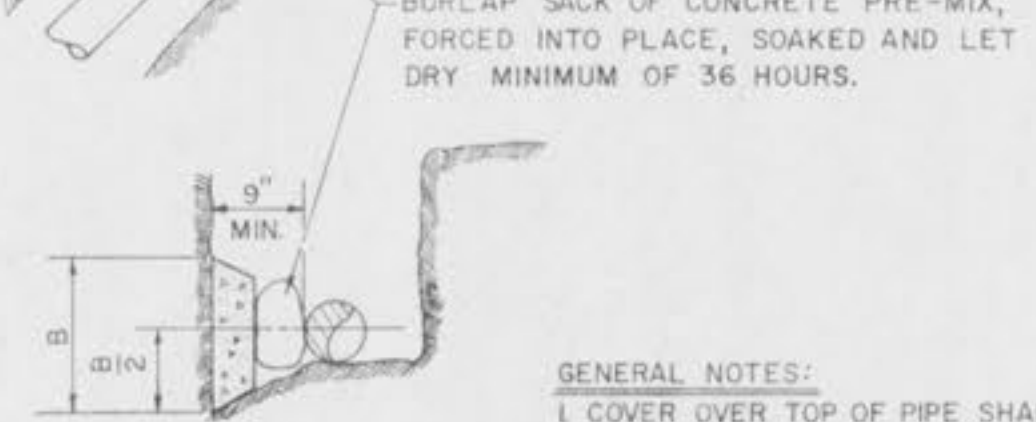
DETAILS THRUST BLOCK FOR HORIZONTAL OFFSETS
