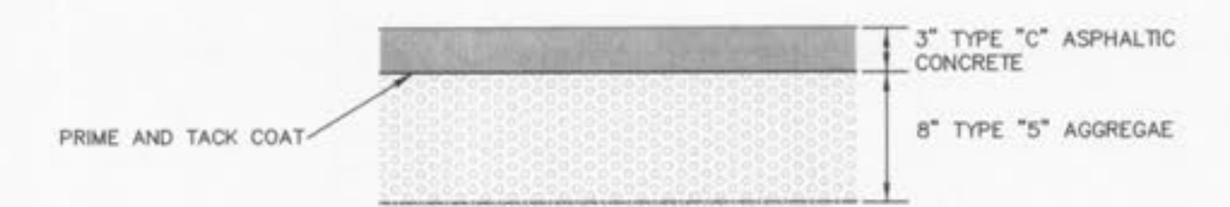
ASPHALT PAVEMENT DETAIL
