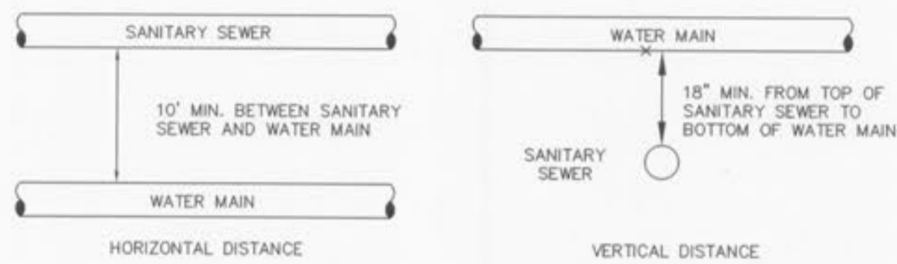
TYPICAL WATER AND SEWER SEPARATION NOT TO SCALE
