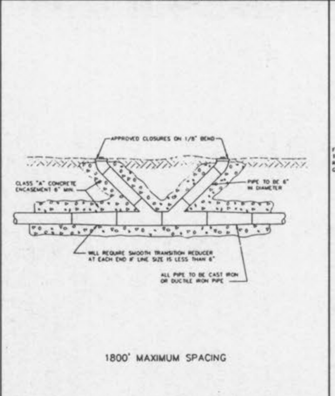
FORCE MAIN CLEANOUT (6" DIA. & SMALLER) METROPOLITAN ST. LOUIS SEWER DISTRICT Standard Details of Sewer Construction Dr. R.C.W. J.C.K. 1992 SHEET 65
