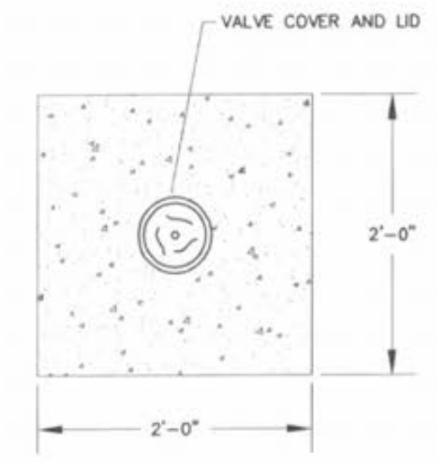
TOP VIEW CONCRETE COLLAR NOT TO SCALE
