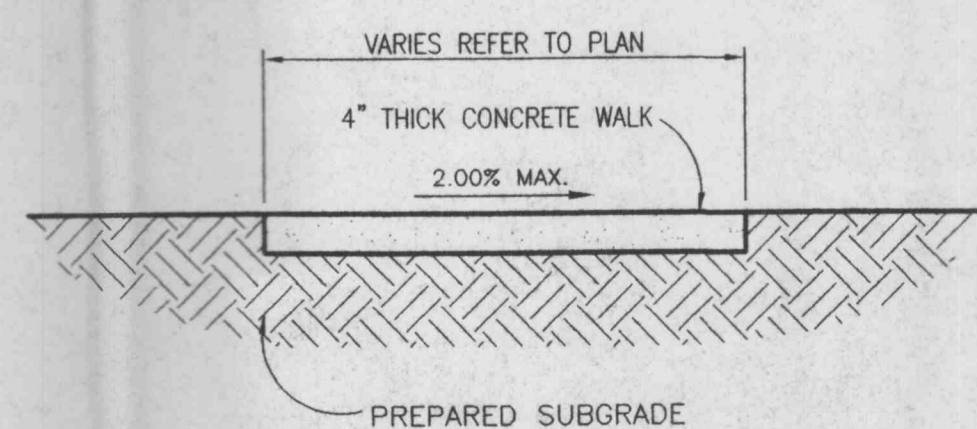
CONCRETE WALK DETAIL NO SCALE
