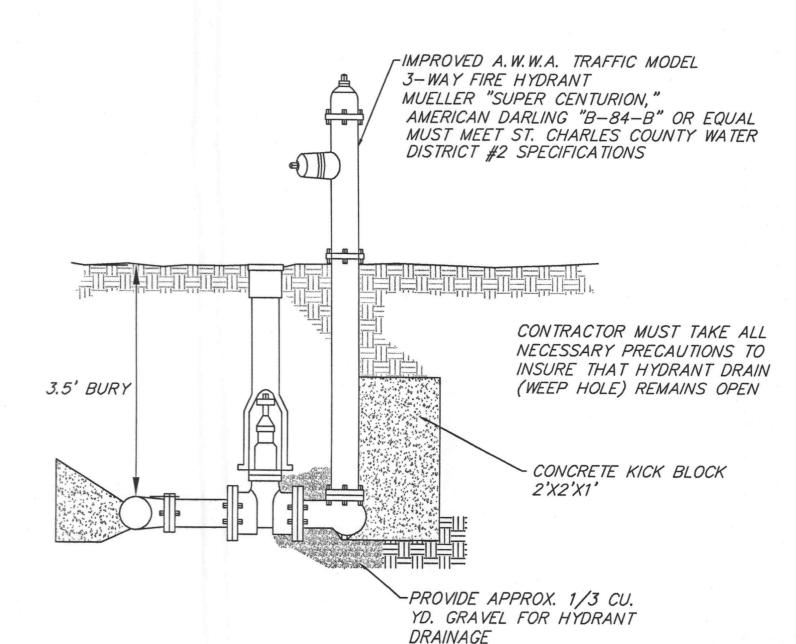
FIRE HYDRANT INSTALLATION DETAIL
