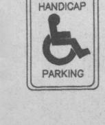
STANDARD 12"X18"X0.080" ALUMINUM 'HANDICAP PARKING' SIGN FACE WITH WHITE LETTERS ON BLUE BACKGROUND (OR LOCALLY APPROVED EQUAL). GALVANIZED STEEL POST 9'-6" LONG. SET BOTTOM OF SIGN 5'-0" ABOVE GRADE. SET BOTTOM OF POST 3'-0" BELOW GRADE.
