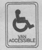
STANDARD 12"X18"X0.080" ALUMINUM 'VAN ACCESSIBLE HANDICAP PARKING' SIGN FACE WITH WHITE LETTERS ON BLUE BACKGROUND (OR LOCALLY APPROVED EQUAL). GALVANIZED STEEL POST 9'-6" LONG. SET BOTTOM OF SIGN 5'-0" ABOVE GRADE. SET BOTTOM OF POST 3'-0"
