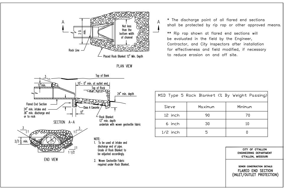
ALL DOWNSTREAM FLARED END SECTIONS REQUIRE A 3 FOOT DEEP CUTOFF WALL AS REQUIRED FOR FE 100 AND FE 102..
