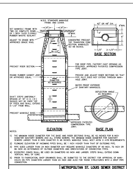
PRECAST CONCRETE MANHOLE
