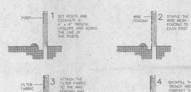
4 BACKFILL THE TRENCH AND COMPACT THE FENCING AND EXCAVATED SOIL EXTEND IT INTO COMPACTED -THE TRENCH BACKFILL 1. FILTER BARRIERS SHALL BE INSPECTED IMMEDIATLY AFTER EACH RAINFALL AND AT LEAST
