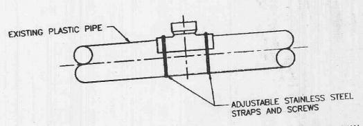
WHEN CONNECTION TO A PLASTIC PIPE IS ALLOWED AND A CONNECTION IS LARGER THAN 6" IN DIAMETER. A SOLVENT WELD WYE OR TEE FITTING OF A SIMILAR MATERIAL MUST BE USED.
