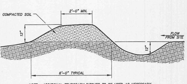
NOTE: ADDITIONAL TEMPORARY DITCHES TO BE USED AS NECESSARY TO CONTROL RUN-OFF. TEMPORARY DIVERSION DITCH
