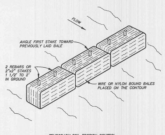
TEMPORARY SOIL EROSION CONTROL STRAW BALE DITCH CHECK NOT TO SCALE
