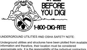
information and therefore, their location must be considered approximate only. It is the responsibility of the individual contractors to notify the utility companies before actual construction. All O.S.H.A rules and regulations established for the type of construction required by these plans shall be strictly followed (ie. trenching, blasting, etc.)
