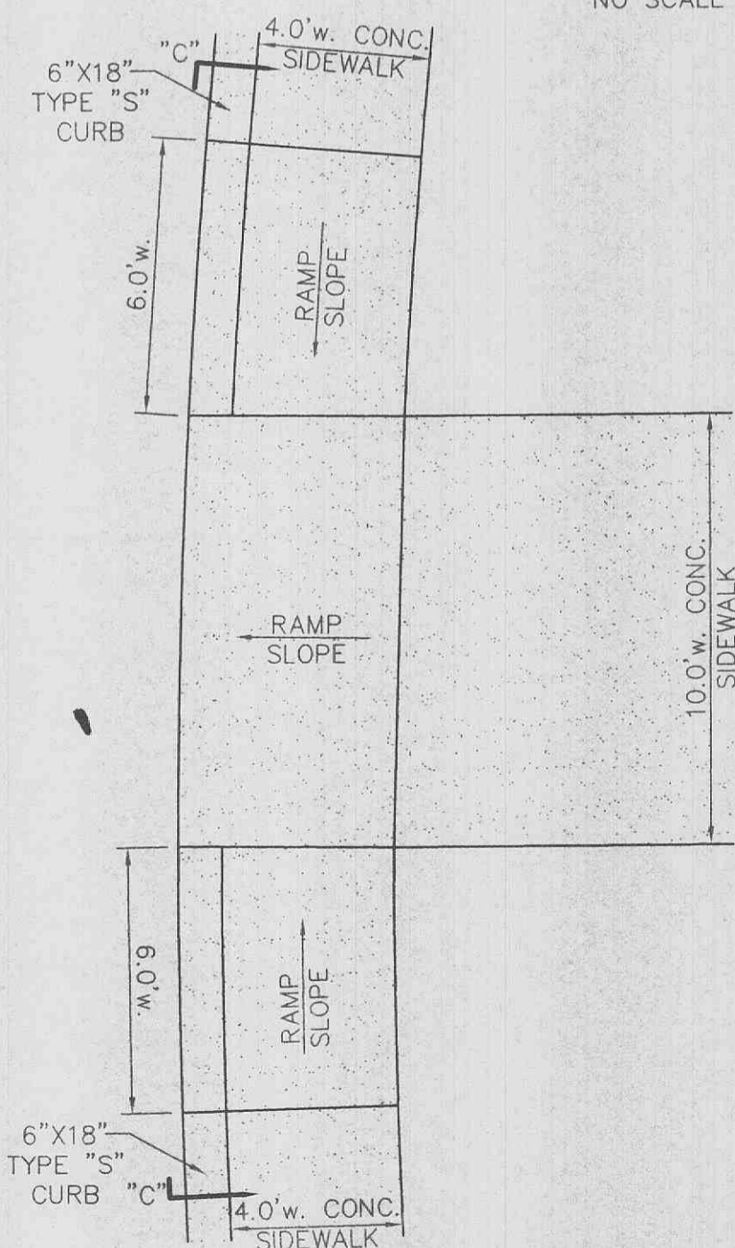
DETAIL "C" AT HANDICAP RAMP NO SCALE
