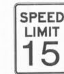
R2-1 "SPEED LIMIT 15" SIGN
