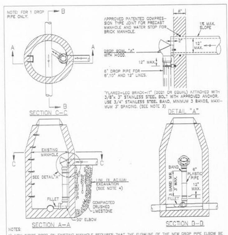
1) NEW INSIDE DROP ON EXISTING MANHOLE REQUIRES THAT THE FLOWLINE OF THE NEW DROP PIPE ELBOW BE CONSTRUCTED AT THE SAME ELEVATION AS THE SPRINGLINE OF THE EXISTING SEWER MAIN AT THE CENTER OF THE EXISTING MANHOLE.
