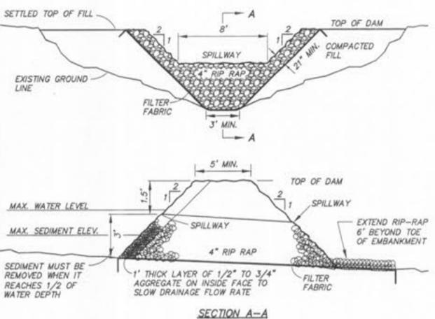
1. SEDIMENT REMOVED FROM STRUCTURE SHALL BE DISPOSED OF AS DIRECTED BY OWNER.
