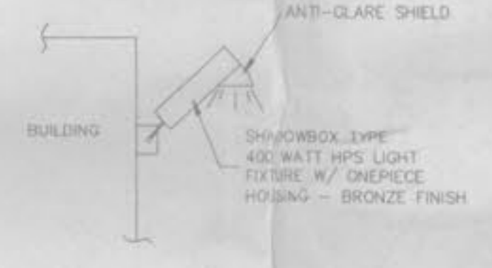
BUILDING MOUNTED LIGHT NOT TO SCALE
