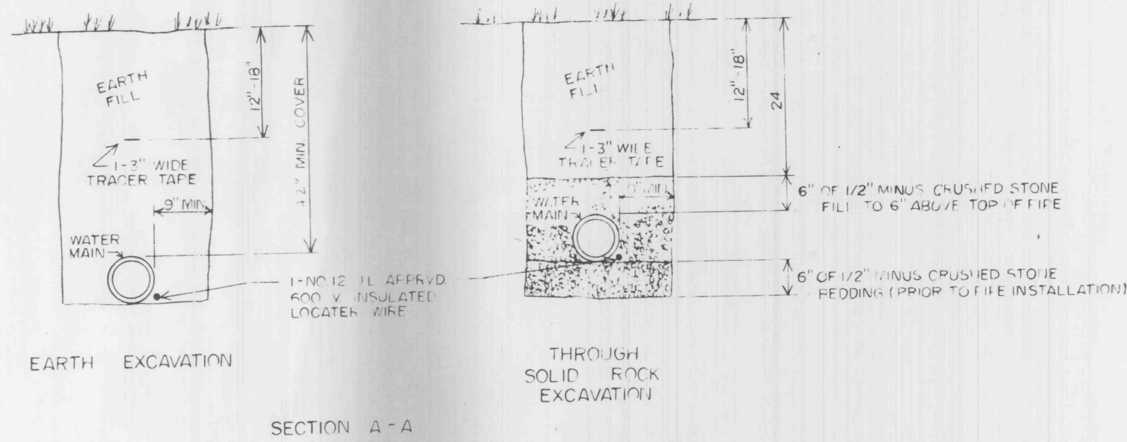
TYPICAL WATER MAIN INSTALLATION DETAILS NO SCALE
