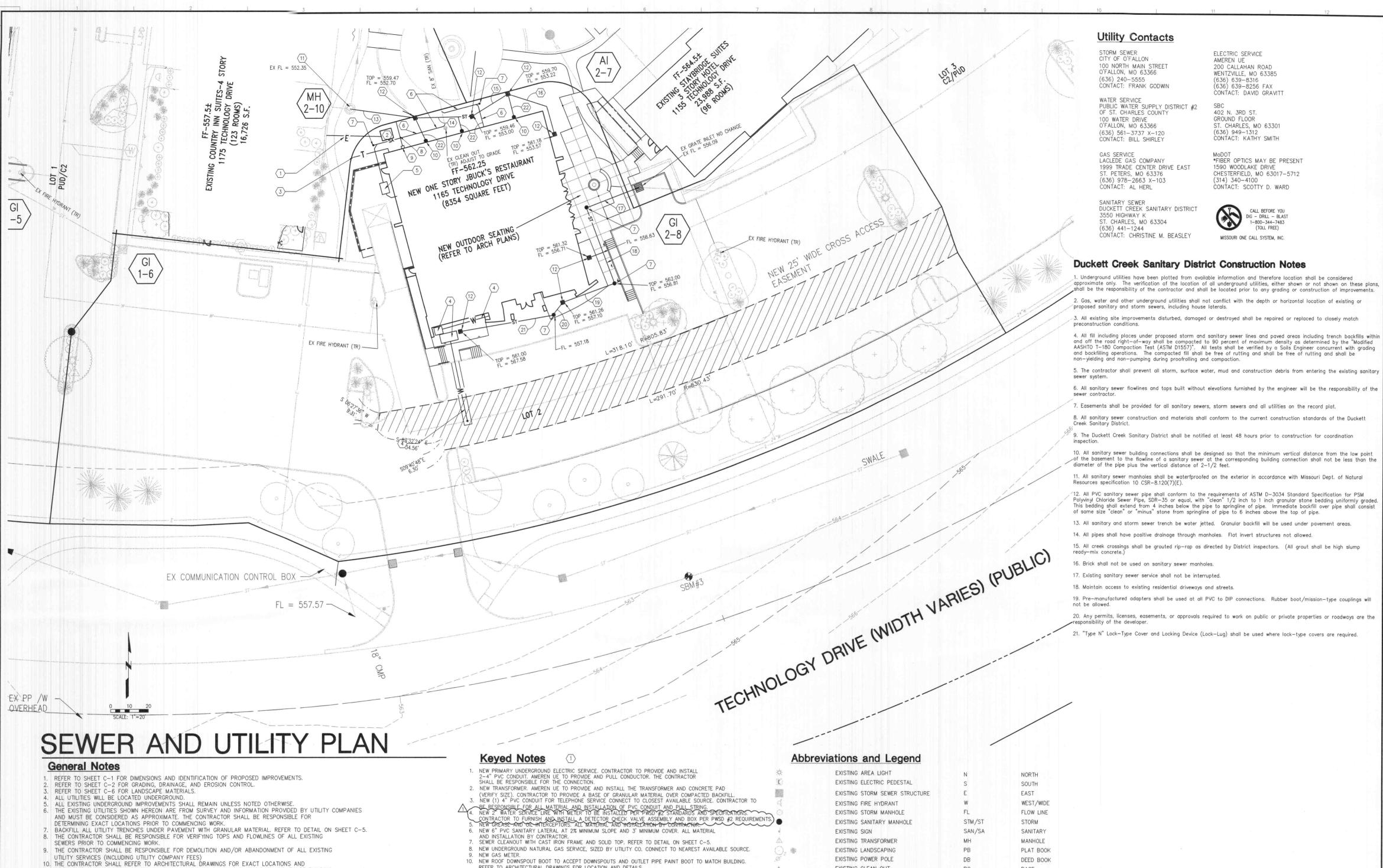
This bedding shall extend from 4 inches below the pipe to springline of pipe. Immediate backfill over pipe shall consist of same size "clean" or "minus" stone from springline of pipe to 6 inches above the top of pipe. 13. All sanitary and storm sewer trench be water jetted. Granular backfill will be used under pavement areas. 14. All pipes shall have positive drainage through manholes. Flat invert structures not allowed.
