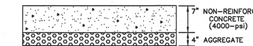
CONCRETE PAVEMENT DETAIL (FOR USE AT ENTRANCES AND TRASH ENCLOSURE PADS AS INDICATED ON PLAN)
